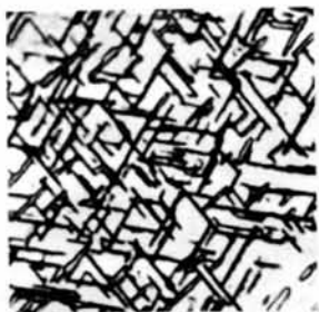
Fig. 1. Micrograph of aluminum-20% silver alloy aged 25½ hr. at 387° C. \times 1300. Resolved cross-sections of precipitate plates are aligned in four orientations relative to the matrix single crystal.
